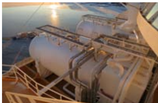
Top view of LNG Tanks mounted on the stern of Viking Grace
